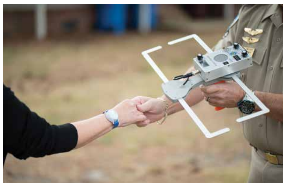
Project Lifesaver radio-frequency tracking device
